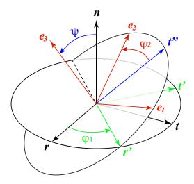
FIGURE 1. Illustration of reference (r, t, n) = (RD, TD, ND) and rotated  $(e_1, e_2, e_3)$  frames using  $(\varphi_1, \psi, \varphi_2)$  Euler angles and Bunge rotation rules.
