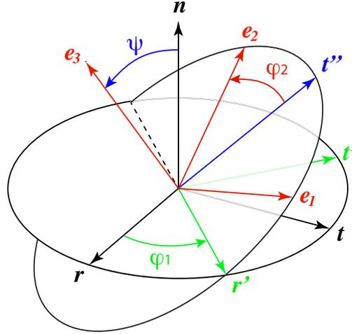
FIGURE 1. Illustration of reference  $(\mathbf{r}, \mathbf{t}, \mathbf{n}) = (RD, TD, ND)$  and rotated  $(\mathbf{e}_1, \mathbf{e}_2, \mathbf{e}_3)$  frames using  $(\varphi_1, \psi, \varphi_2)$  Euler angles and Bunge rotation rules.
