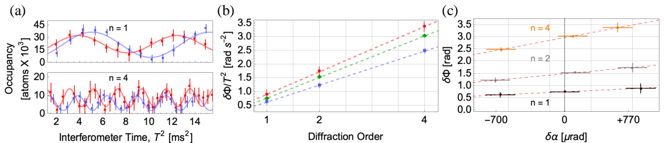
FIG. 4. Demonstrating inertial sensitivity. (a) Fringe pattern obtained from three pulse Bragg interferometers by scanning the dwell time T of the interferometer. Results are shown for n = 1 and 4 using two different angles \alpha (red and blue). Each data point represents an average of 20 measurements. (b) Scale factor of the atom interferometer as a function of the diffraction order for three different tilts \alpha , normalized to T = 1 second. The fringe patterns from a) correspond to the points for n = 1 and 4 , in red and blue. We applied different tilts to the experiment, extracted from the fits as 2203 \pm 8 \mu\text{rad} (red), 1378 \pm 8 \mu\text{rad} (green), and 620 \pm 7 \mu\text{rad} (blue). (c) Inertial sensitivity of the atom interferometer as a function of the tilt angle, separated by diffraction order, normalized to T = 1 second. The dashed red lines are calculated \delta\Phi for each diffraction order n .
