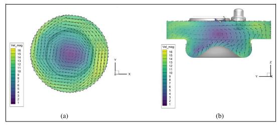
**Figure 3.** Example of 2D flow-field (m/s) in a SACI engine at 37 CAD BTDC – 1000 rpm: (a) horizontal cut at middle distance between the cylinder head and the bowl and (b) vertical cut at central line of the chamber (perpendicular to the intake and outlet lines).
