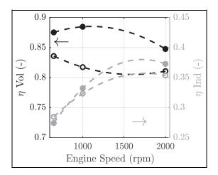
**Figure 11.** Volumetric and indicated efficiencies as function of engine speed – CR = 17:1,  $\phi$  = 1, Pin = 1 bar, Tin = 50°C. Empty symbol = SI engine with 10% H<sub>2</sub>.
