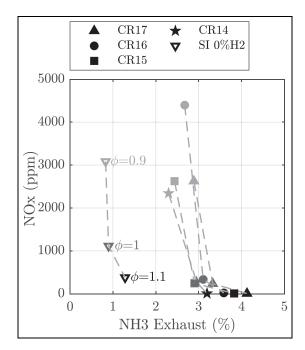
Figure 15.  $NO_x$  -NH<sub>3</sub> emission 1 bar as a function of CR - 1000 rpm, Pin = 1 bar.
