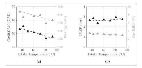
**Figure 8.** (a) Combustion duration and specific consumption and (b) IMEP and stability as a function of the intake temperature- $\phi = 1$ , 1500 rpm, Pintake = 0.5 bar in SACI.
