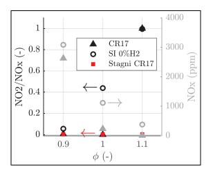
**Figure 17.** NO<sub>2</sub>/NO<sub>x</sub> ratio and NO<sub>x</sub> emissions as a function of equivalence ratio – 1000 rpm, Pin = 1 bar and CR 17:1. Comparison with NO<sub>2</sub>/NO<sub>x</sub> ratio values predicted by kinetics simulation with the STAGNI mechanism at 100 CAD ATDC.
