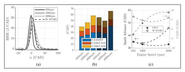
**Figure 6.** (a) Heat release rate, (b) combustion duration, and (c) combustion phasing for different engine speeds -data in SI with 10% H<sub>2</sub>- $\phi$  = 1, CR = 17, Pin = 1 bar, Tin = 50°C. Shaded bars for SI engine.
