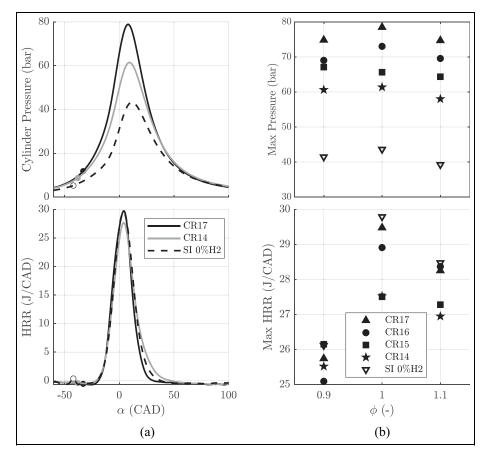
**Figure 4.** (a) In-cylinder pressure and heat release rate for stoichiometric ammonia/air mixture at CR = 14 and 17, bullet correspond to SIT and (b) max heat release rate and in-cylinder pressure for 4 CR and 3 equivalence ratios Data from SI (0%H2, CR = 10.5:1) – 1000 rpm, Pin = 1 bar, Tin = 50°C.
