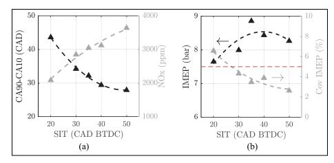
Figure 7. (a) Combustion duration and NO<sub>x</sub> emissions and (b) IMEP and COV<sub>IMEP</sub> $\Rightarrow$  = 0.85, 1500 rpm, 1.08 bar, SACI CR 17:1 and SIT = 40 CADBTDC.
