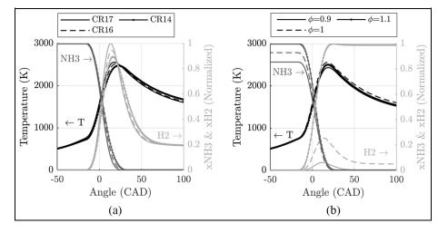
**Figure 14.** Evolution of average chamber temperature and NH<sub>3</sub> and H<sub>2</sub> fractions estimated by kinetics simulation using Stagni mechanism: (a) for different CR at  $\phi = 1$  and (b) for different equivalence ratios at CR = 17:1.
