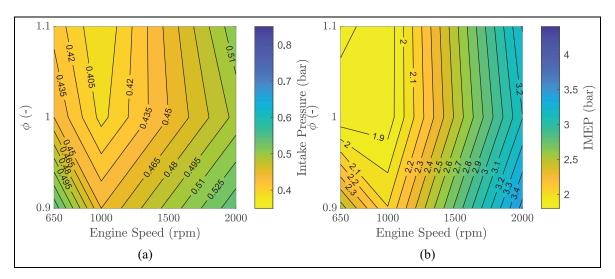
**Figure 10.** (a) 2D plot of minimim intake pressure limit and (b) 2D plot of corresponding IMEP as a function of engine speed and equivalence ratio - CR = 17:1, Tin = 50°C, Pin = 1 bar.
