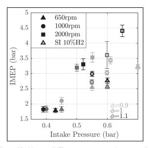
**Figure 12.** Minimum IMEP versus minimum intake pressure for three engine speeds - CR = 17:1, Tin = 50°C. Previous data in SI engine with 10% H<sub>2</sub>.
