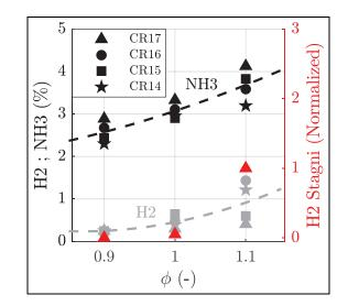
Figure 13. Ammonia and hydrogen exhaust emissions at 1000 rpm for different CR – comparison with  $H_2$  values predicted by kinetics simulation with the STAGNI mechanism at 100 CAD ATDC.
