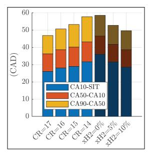
**Figure 5.** Combustion duration analysis as a function of the compression ratio. Shaded bars for SI engine with different H2% content – 1000 rpm,  $\phi = 1$ , Pin = 1 bar, Tin = 50°C.
