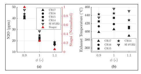
Figure 16. (a)  $N_2O$  emissions as a function of equivalence ratios for different CR - 1000 rpm, Pin = I bar – values from kinetics simulation at CR 17:1 at 100 CAD ATDC and (b) exhaust temperature as a function of equivalence ratio for all CR - 1000 rpm, Pin = I bar.
