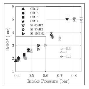
Figure 9. Minimum IMEP versus minimum intake pressure at 1000 rpm – Tin = 50°C.
