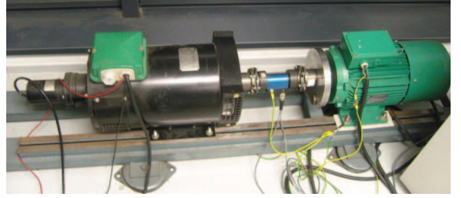
Fig. 6. Experimental test bench composed of a 5.5 kW induction machine (right), a direct current motor to produce the load torque (left) and a iron disk placed on the shaft to create the different levels of mechanical unbalance.
