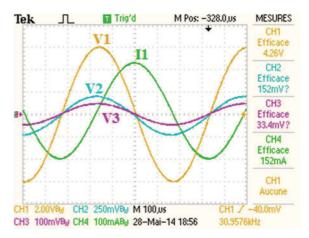
Fig. 7. Voltage V1 (CH1), induced voltages V2 (CH2), V3 (CH3) and current I1 (CH4)
