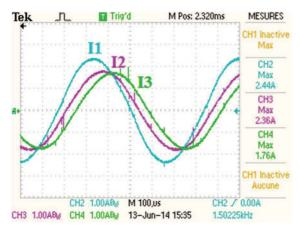
Fig. 6. Inductor currents in phases 1, 2 and 3
