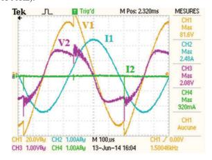
Fig. 8. Phase 1 and 2 voltages and currents during the identification step on phase 1 with modulated angle on inverter 1 and phases 2 and 3 open circuited. CH1:V1; CH2:I1; CH3:V2 and CH4:I2
