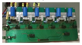
Fig. 4. The 6-phase voltage inverter
