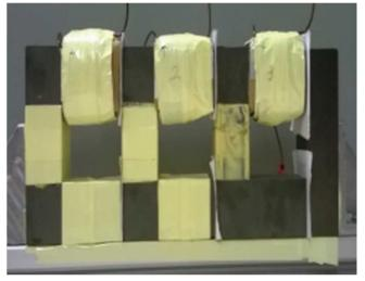
Fig. 2. Three coupled coils
