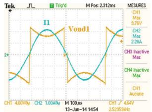
Fig. 5. Inverter 1 output voltage and current
