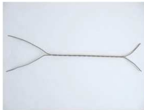
Figure 5. Enameled wire PEI-PAI thermal class: 200°C
