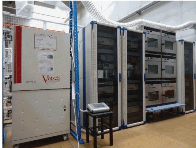
Figure 2. The experimental setup for accelerated tests
