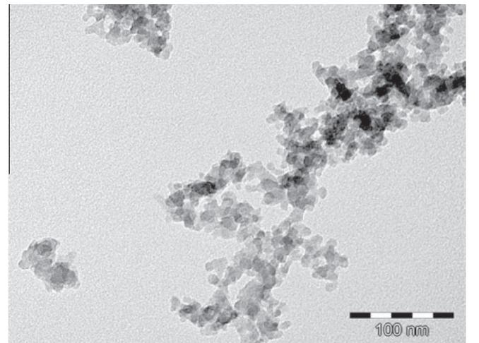
**Fig. 1.** Typical TEM micrograph of S1 dispersion reveals a branched structure made of connected clusters composed of small silica beads welded together into larger dense areas.
