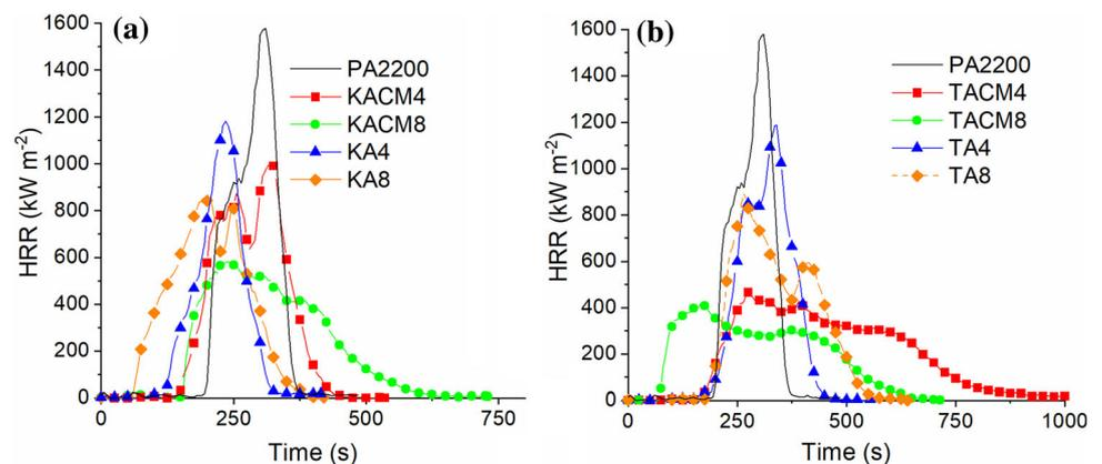
**Table 4** Cone calorimeter results of formulations containing coated and uncoated kaolin and talc
