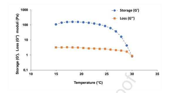
Figure 10. Measurement of storage and loss moduli as f. nction of the temperature.
