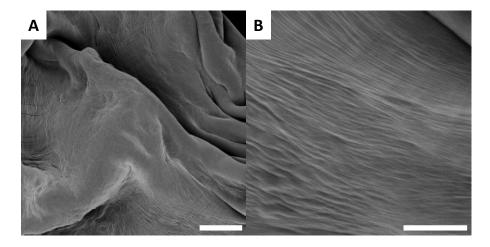
**Figure 12.** SEM images of the dried hydrogel (Scale bar, A: 10, μm and B: 30 μm).
