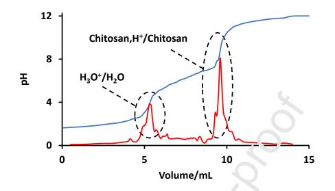
**Figure 5.** Example of titration curve for *Helio*  $o_{\mu}$  *ric dilloni* chitosan deacetylation degree determination (Blue: titration curve and rd: first derivative of the titration curve).
