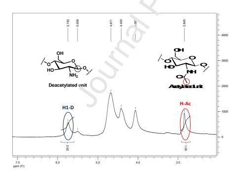
Figure 4. Example of <sup>1</sup>H NMR for *Heliocopris dilloni* Chitosan.
