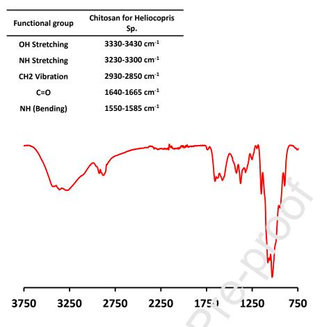
Figure 3. FT-IR spectrum of *Heliocopris* s<sub>1</sub> chitosan.
