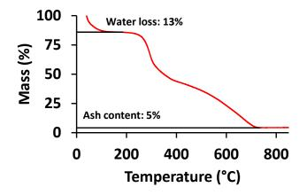
Figure 7. TGA curve for Heliocopris dilloni chitosan.
