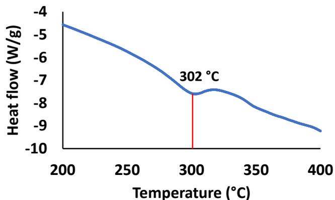
**Figure 6.** DSC observation for *Heliocoprís dilloni* chitosan.
