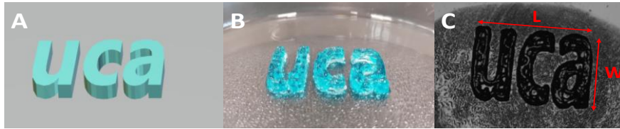
Figure 14. Evaluation of the printing accuracy. A: Theoretical model, B: Printed shape and C: measurement.
