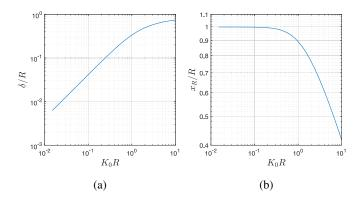
Figure 8: Evolution of the deflection  $y(x_R) = \delta$  (a) and the radial extension  $x_R$  (b), see equation 4.3, as function of the curvature  $K_0$ .
