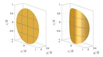
Figure 3: 3D representation of an undistorted disc  $K_0 = 0$ , on the left, and of a bent disc,  $K_0 R=1$ , on the right.
