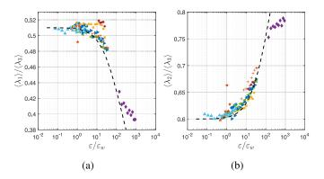
Figure 7: Evolution of the mean shape factors  $\langle \lambda_1 \rangle / \langle \lambda_3 \rangle$  (a) and  $\langle \lambda_2 \rangle / \langle \lambda_3 \rangle$  (b) as a function of the normalised turbulent dissipation rate  $\varepsilon / \varepsilon_r$ . The dashed line represents the best fit of an ideal bent disc, *cf*. text for more details.
