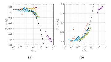
Figure 5: Evolution of the mean shape factors  $\langle \lambda_1 \rangle / \langle \lambda_3 \rangle$  (a) and  $\langle \lambda_2 \rangle / \langle \lambda_3 \rangle$  (b) as a function of the normalised turbulent dissipation rate  $\varepsilon / \varepsilon_v$ . The dashed line represents the best fit of an ideal bent disc, see text for more details.
