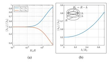
Figure 4: a) Theoretical evolution of the shape factors of a bent disc represented on Figure 3 as a function of the normalised curvature  $K_0R$ . b) Evolution of the mean shape factor  $\langle \lambda_2 \rangle / \langle \lambda_3 \rangle$  for a partially empty cylinder.
