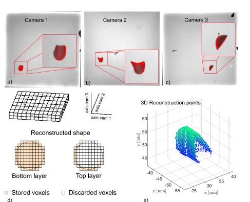
Figure 1: a,b and c) Typical images with a superimposition of the reconstructed disc shown in red dots. d) Illustration of the reconstruction process with the voxel selection. Here for simplicity, the axis of the voxel array is aligned with the axes of the cameras. e) Reconstructed object from the convex hull volume method with the voxel selection detailed in the text. The color codes the *z* coordinate of the voxel
