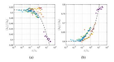
Figure 6: Evolution of the mean shape factors  $\langle \lambda_1 \rangle / \langle \lambda_3 \rangle$  (a) and  $\langle \lambda_2 \rangle / \langle \lambda_3 \rangle$  (b) as a function of the normalised turbulent dissipation rate  $\varepsilon / \varepsilon_r$ . The dashed line represents the best fit of an ideal bent disc, *cf*. text for more details.
