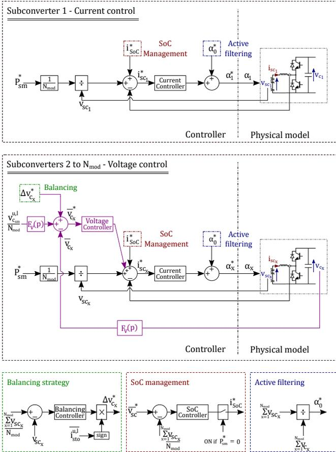
Fig. 6: Control architecture of the modular interface converter
