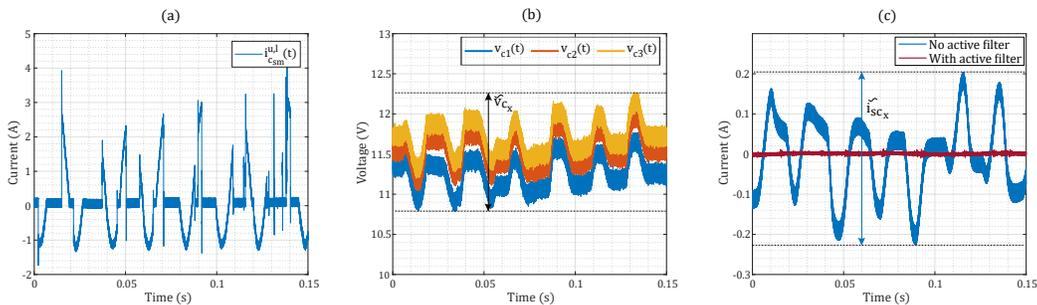
Fig. 11: Experimental results during normal operation ( $P_{sm} = 0$ ) with: (a) ES-SM capacitor current (b) Intermediate capacitance voltage of each subconverter (c) Supercapacitor stack current
