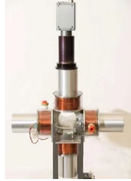
Figure 12. Electromagnetic coil setup consisting of six coils. Two of four horizontal coils are removed to allow viewing of workspace. [92].
