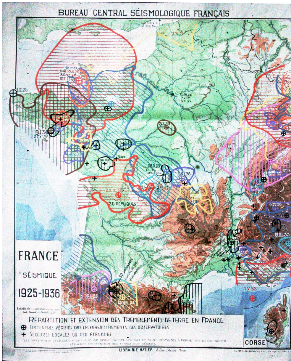
Figure 16. Map of the distribution and extension of earthquakes in France. The different colours do not have any special meanings and are intended to make it possible to distinguish the areas of the extensions of the main earthquakes for the years 1925–1936. [Rothé, 1937] (with gracious authorization of Hatier edition).
