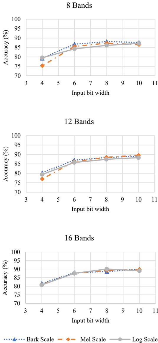
Fig. 6. Accuracy of the full-resolution network as a function of the input bit width according to different number of bands. The values are extracted as the best accuracy found over multiple trainings. The best value obtained during training is 90.02% with 16-channel and 8-bit input quantization.
