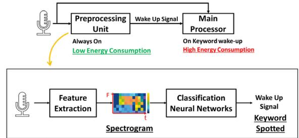
Fig. 1. Typical architecture of a preprocessing unit
