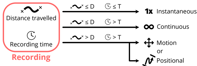
Figure 5: The design tool infers the spatio-temporal mapping of a vocalization directly after recording by considering the user’s movement magnitude and the recording duration. D (0.5 m) and T (2.5 s) are empirically determined constants.
