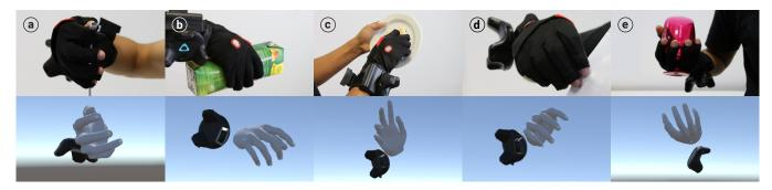
Figure 9: Proof-of-concept system using VR glove hardware supporting five frequently used grasps. (a) Charge Cell Phone, (b) Pour Juice Bottle, (c) Scratch Sponge, (d) Take Letter from Envelope, and (e) Toast Wine. The screenshots show the Unity hand model.
