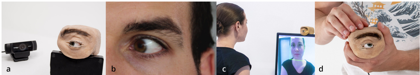
Figure 1: a) Eyecam is an alternative anthropomorphic design of conventional webcams, b) which draws inspiration from the human eye morphology to c) exaggerate the sensing capacities of webcams like face detection, and d) foster affective relationships.
