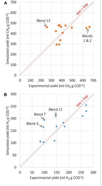
FIGURE 2 | Simulated and experimental biogas production yields: (A) anaerobic digestion (AD); (B) dark fermentation (DF).
