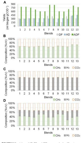
**FIGURE 3** | Simulations of AD, DF, and ADF processes for the different substrate blends: **(A)** Total biogas production yields for AD, DF, and ADF; **(B)** Biogas composition for AD; **(C)** Biogas composition for DF; **(D)** Biogas composition for ADF.
