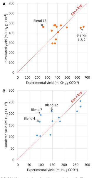
FIGURE 2 | Simulated and experimental biogas production yields: (A) anaerobic digestion (AD); (B) dark fermentation (DF).
