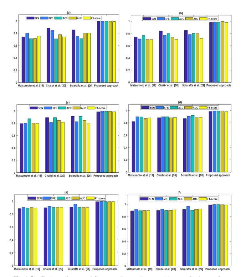
**Fig. 4.** Classification performance of the proposed approach compared to conventional ones using simulated data for different SNR values: (a): -10 dB, (b): -5 dB, (c): 0 dB, (d): 5 dB, (e): 10 dB and (f): 15 dB.
