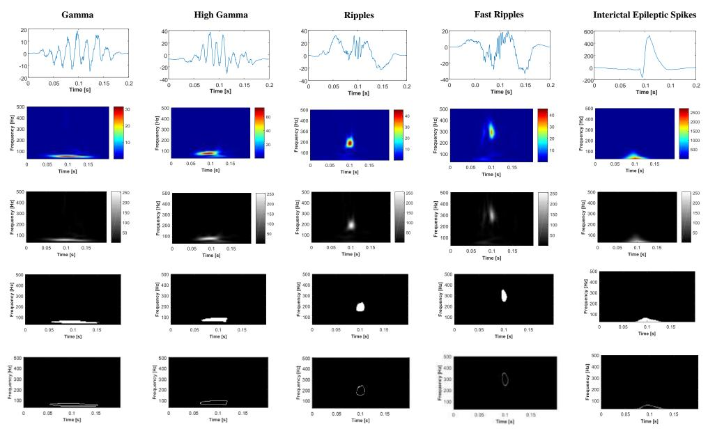
**Fig. 2**. Representation of HFOs and IESs patterns in time domain (first row) (i) TF plane (second row), (ii) TF based grayscale image (third row), (iii) binarized TF based grayscale image (fourth row) and (iv) TF based grayscale image gradient (fifth row).
