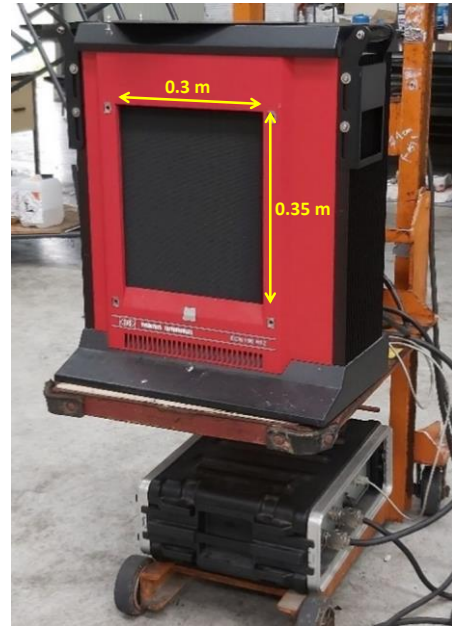
Figure 6 A photo of the electric black body used in the experiments. The control box underneath makes it possible to adjust the surface temperature and the internal ventilation of the black body equipment.
