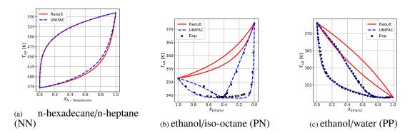
Figure A.3: Boiling-point diagrams for three mixtures with different polarity behaviors at 1 atm. The experimental data presented in (b) and (c) are extracted from [47] and [48], respectively.
