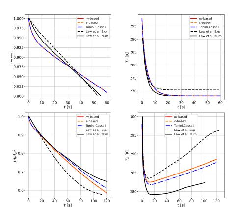
Figure A.8: Comparison of modeling approaches through normalized droplet surface and temperature evolution for a pure Methanol droplet with relative air humidity phi = 0.0 (top) and  $\phi = 1.0$  (bottom)
