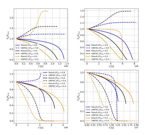
Figure A.7: Comparison of VLE approaches through normalized Ethanol mass fraction inside the droplet for a ethanol/iso-octane (top) and ethanol/water (bottom) droplets with initial diameter  $d_0 = 50\mu m$ , initial temperature  $T_{d,0} = 304K$ , surrounding gas temperature  $T_{\infty} = 304K$  (left figures) and  $T_{\infty} = 703K$  (right figures) and varying initial compositions.
