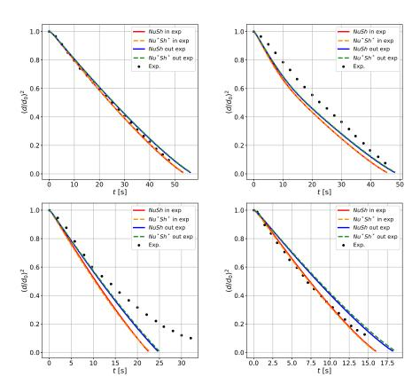
Figure A.12: Normalized droplet surface and temperature for varying initial compositions ( $VF_{Eth}=0$ ,  $VF_{Eth}=0.25$ ,  $VF_{Eth}=0.75$ ,  $VF_{Eth}=1.0$  left-to-right, top-to-bottom) of a ethanol/water droplet of initial diameter  $d_0=1.2mm$  and temperature  $T_{d,0}=293.15K$  with surrounding gaseous temperature  $T_{\infty}=400K$
