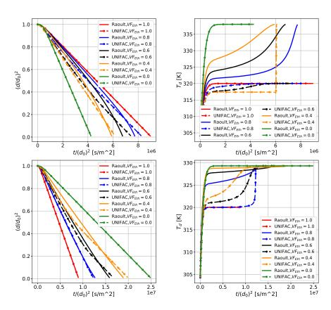
Figure A.6: Comparison of VLE approaches through normalized droplet surface and temperature evolution for a ethanol/iso-octane (top) and ethanol/water (bottom) droplets with initial diameter  $d_0 = 50\mu m$ , initial temperature  $T_{d,0} = 304K$ , surrounding gas temperature  $T_{\infty} = 703K$  and varying initial compositions.
