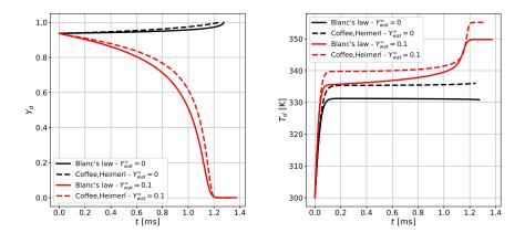
Figure A.11: Ethanol composition inside droplet and droplet temperature for a VF=0.95 ethanol/water droplet of initial diameter  $d_0=20\mu m$  and temperature  $T_{d,0}=300K$  with surrounding gaseous temperature  $T_{\infty}=1500K$  and water mass fraction at infinity  $Y_{wat}^{\infty}=0.0$  and  $Y_{wat}^{\infty}=0.1$
