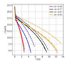
Figure A.13: Droplet instantaneous radius for a 50% ethanol, 50% water (mass fractions) droplet of initial radius  $d_0 \approx 22 \mu m$  and temperature  $T_{d,0} = 293 K$  with surrounding gas temperature  $T_{\infty} = 293 K$  and various relative humidities representing water vapor at infinity. Depicted are the current model proposition (continuous lines) and the data from Gregson et al. [37] (dashed lines for experimental data, dot-dash lines for numerical results)
