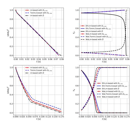
Figure A.10: Normalized droplet surface and internal composition for a VF=0.95 ethanol/water droplet of initial diameter  $d_0=20\mu m$  and temperature  $T_{d,0}=300K$  with surrounding gaseous temperature  $T_{\infty}=300K$  and relative humidity of  $\phi=0.0$  (top) and  $\phi=0.4$  (bottom)
