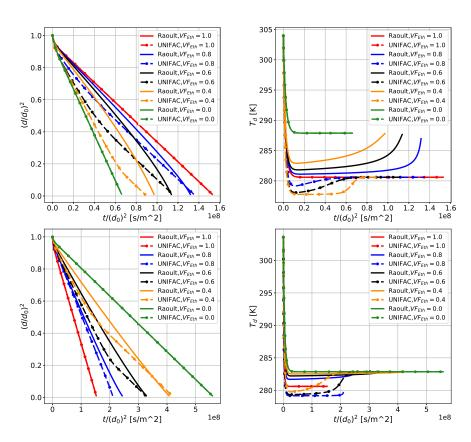
Figure A.5: Comparison of VLE approaches through normalized droplet surface and temperature evolution for a ethanol/iso-octane (top) and ethanol/water (bottom) droplets with initial diameter  $d_0 = 50\mu m$ , initial temperature  $T_{d,0} = 304K$ , surrounding gas temperature  $T_{\infty} = 304K$  and varying initial compositions.
