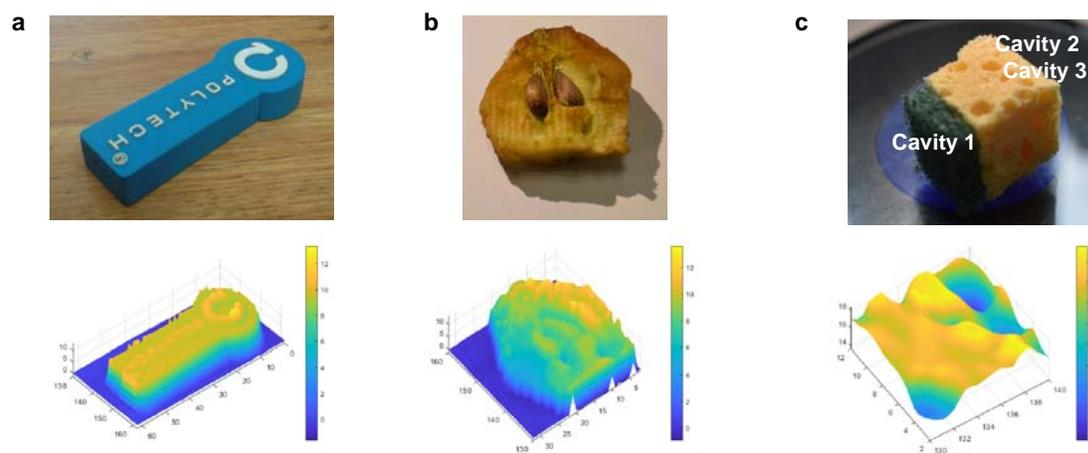
**Fig. 2. Topographical images created using the topography MSI.** Optical and topography maps of **a** USB key, **b** apple core with seeds and **c** 1 cm<sup>2</sup> surface of a sponge piece. The color bars indicate the height differences in mm.
