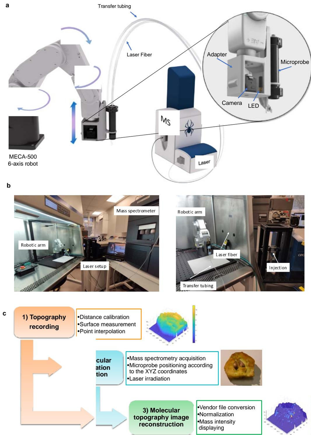
**Fig. 1. Schematic representation of the Robot-Assisted SpiderMass technology and the general workflow of operation.** **a**, The SpiderMass probe is attached with an adaptor to the robotic arm. The zoomed part details the distance sensor system with a separate compartment for the camera and an LED laser pointer. The arrows indicate some degrees of movements of the 6-axis robotic arm. The
