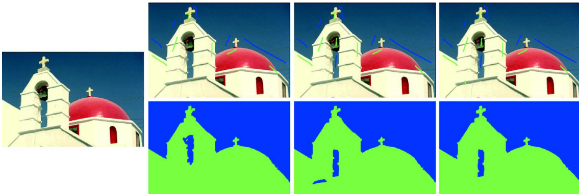
Fig. 12 S \alpha F seed evolution example for a binarization problem. Only two updates of seeds are required to achieve an accurate result.
