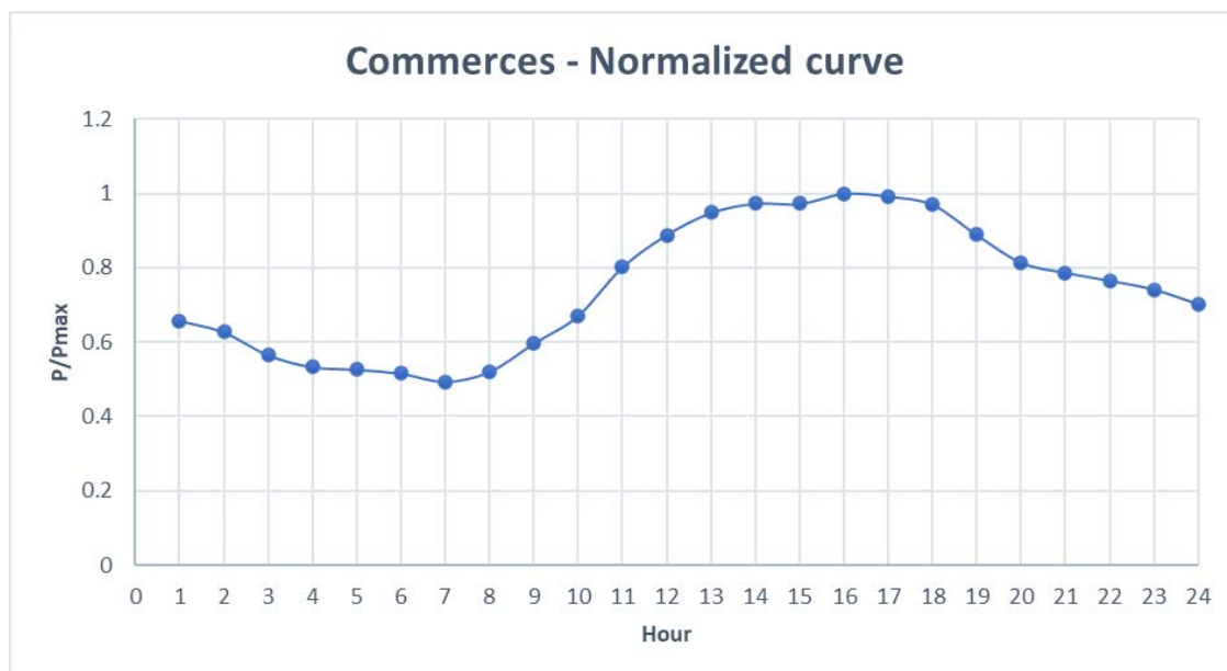
Figure 63. Annual load curve on daily basis used for the tertiary sector (based on Hayes et al., 2013)
