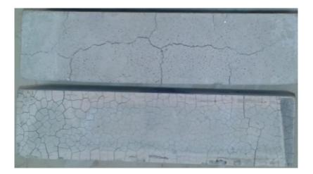
Fig. 5 – Mortars Microcracking beyond 400°C (W/C=0,5 and 0,6)
