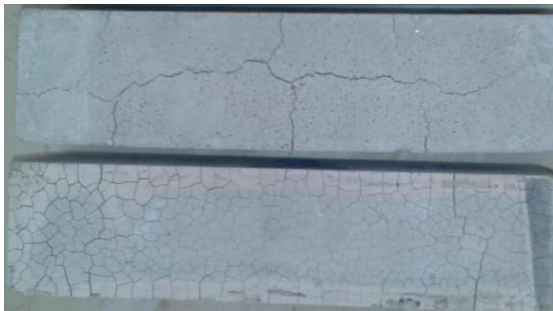
Fig. 5 – Mortars Microcracking beyond 400°C (W/C=0,5 and 0,6)
