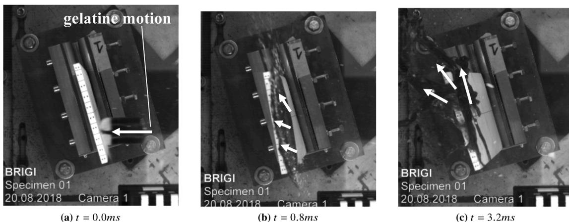
Fig. 26. Experimental gelatine deformation; (a) - (c) show the experimental gelatine behaviour throughout the laminate deflection cycle for the *CP1* test. Gelatine motion is indicated using white arrows.
