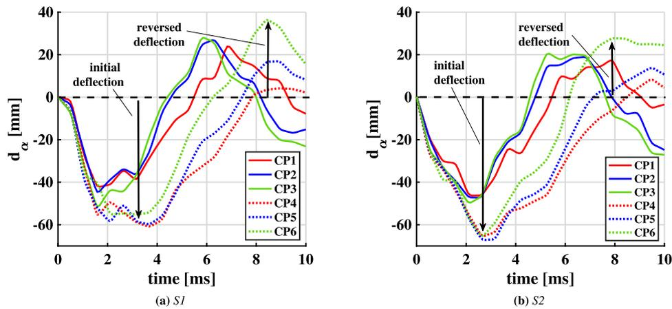
Fig. 18.  $\alpha$  – axis tip displacements from tests CP1 - CP6 on unpinned laminates showing data taken from point S1 (a) and points S2 (b) with points of initial and reversed full deflections highlighted.
