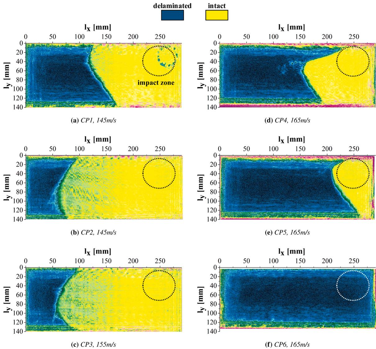
Fig. 23. C-scan plots of delamination for unpinned laminates CP1 - CP6, showing region of impact. The specimen root corresponds to  $l_x = 0\text{mm}$ , the visible edge in HSV1 corresponds to  $l_x = 290\text{mm}$  and the visible edge in HSV2 corresponds to  $l_y = 140\text{mm}$ .
