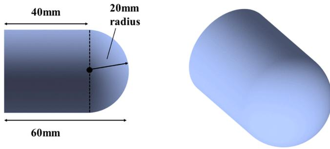
Fig. 7. 'Rounded cylinder' projectile design, showing key dimensions.
