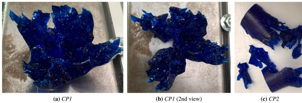
Fig. 17. Retrieved gelatine from cases CP1 (Fig. 17a and b) and CP2 (Fig. 17c), both using a test velocity of  $V_i = 145\text{m/s}$ , showing gelatine damage and intact nature of projectiles post-impact.
