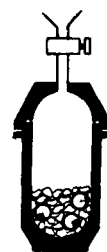
Fig.3. Stainless-steel container used to crush ice samples and recover air from the bubbles.
