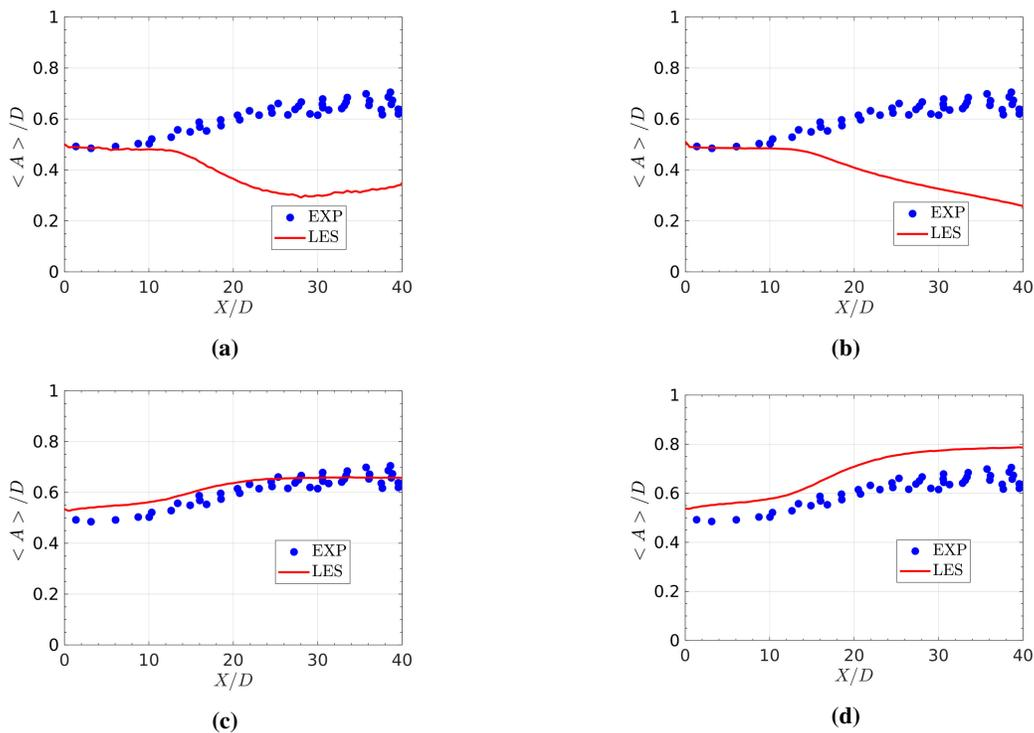
**Fig. 15** Mean jet diameter based on different criteria for the LES : (a)  $max(\|\vec{\nabla}\alpha_l\|)$ , (b)  $\alpha_{limit} = 0.5$ , (c)  $\alpha_{limit} = 0.15$ , (d)  $\alpha_{limit} = 0.1$ .
