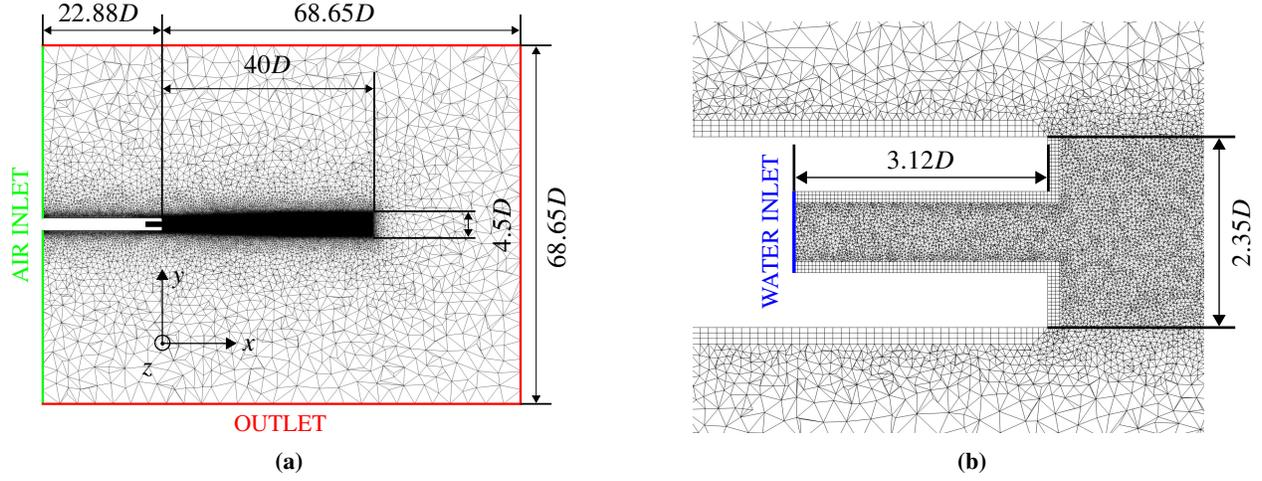
Fig. 2 Mesh representation : (a) full mesh, (b) zoom.
