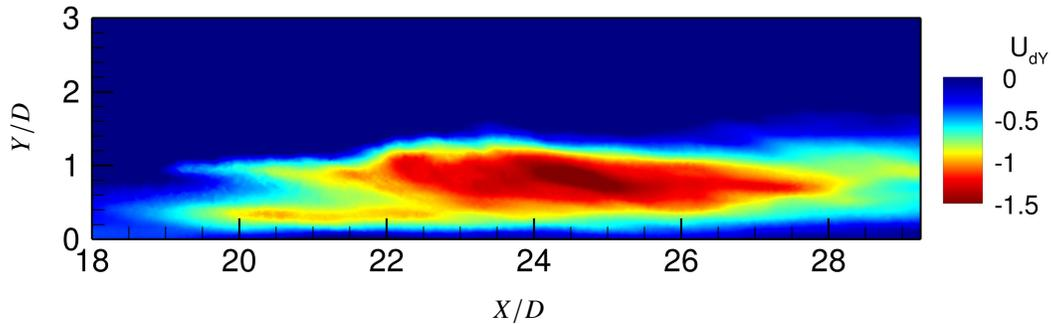
**Fig. 22** Mean values of the droplet velocity  $U_{dY}$  in  $Y$  direction in the plane  $(X, Y)$  [ $\text{m s}^{-1}$ ].
