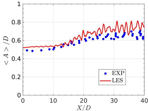
**Fig. 14** Mean radius of the liquid jet.
