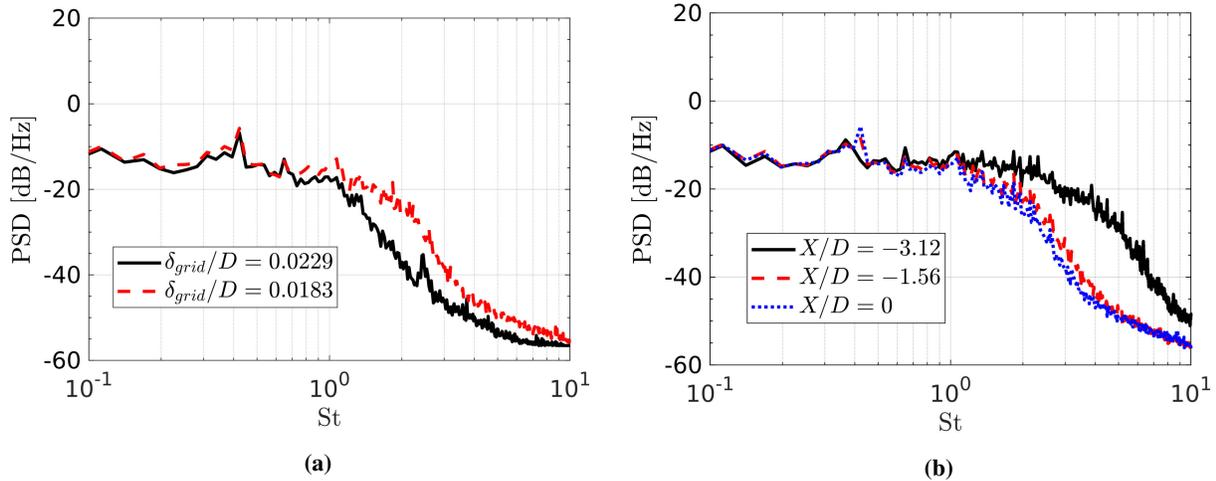
**Fig. 7 Power spectral density of  $U_x$  obtained at  $r/D = 0.4$  using SEM with  $N = 100$  and  $\sigma/D = 10$  : (a) for  $\delta_{grid}/D = 0.0183$ , (b) at  $X = 0$  for  $\delta_{grid}/D = 0.0229$  and  $\delta_{grid}/D = 0.0183$ .**
