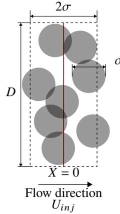
**Fig. 3 Principle of eddy generation with SEM.**
