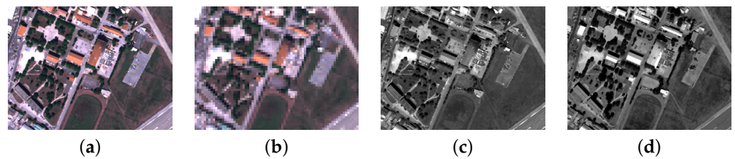
Figure 6. “Toulon” dataset (spatial resolutions in brackets; RGB representation for HS images). (a) REF (1.5 m), (b) HS (6 m), (c) PAN, visible (1.5 m), (d) PAN, SWIR (1.5 m).
