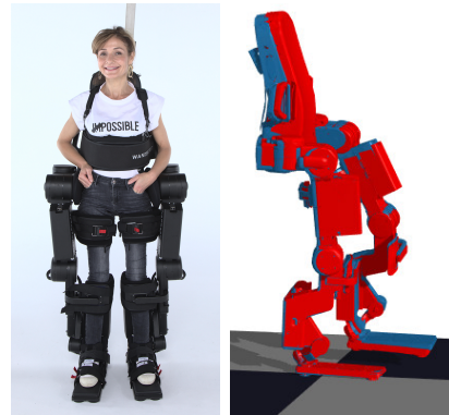
Fig. 1. Picture of the exoskeleton Atalante with a paraplegic user. On the right, CAD reconstruction under the assumption of full rigidity (blue), and ground truth from motion capture (red): the real robot is leaning forward due to deformations.
