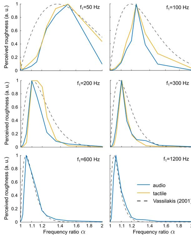
**Fig. 2.** Audio (blue line) and tactile (yellow line) roughness curves obtained from the experiment. The two modalities elicit similar roughness maxima and are coherent with the theoretical auditory roughness model proposed by Vassilakis (2001) (dashed line). The stimuli with  $f_1 = 600$  and  $1200$  Hz were presented only for the audio condition, because they are beyond the frequency bandwidth of tactile perception.
