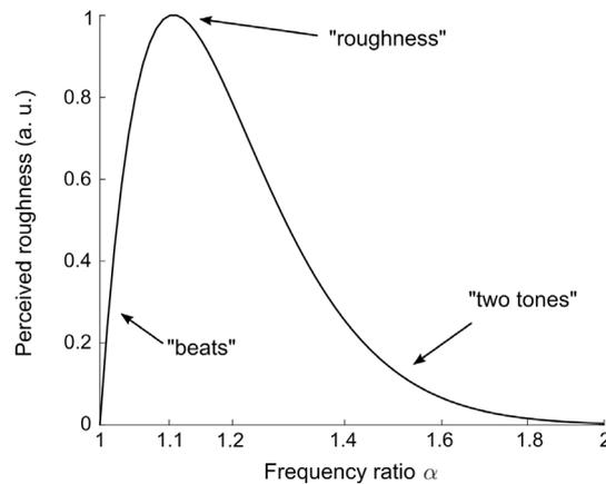
**Fig. 1.** Typical auditory roughness curve of a sum of two monochromatic tones and description of the three kinds of sensations provoked by pairs of pure tones for  $f_1 = 200$  Hz (Vassilakis, 2001).
