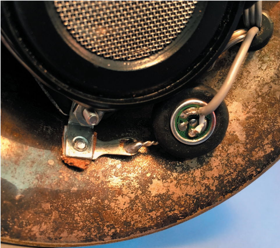
Figure 25. Pressure-zone electret microphone mounted inside bell.
