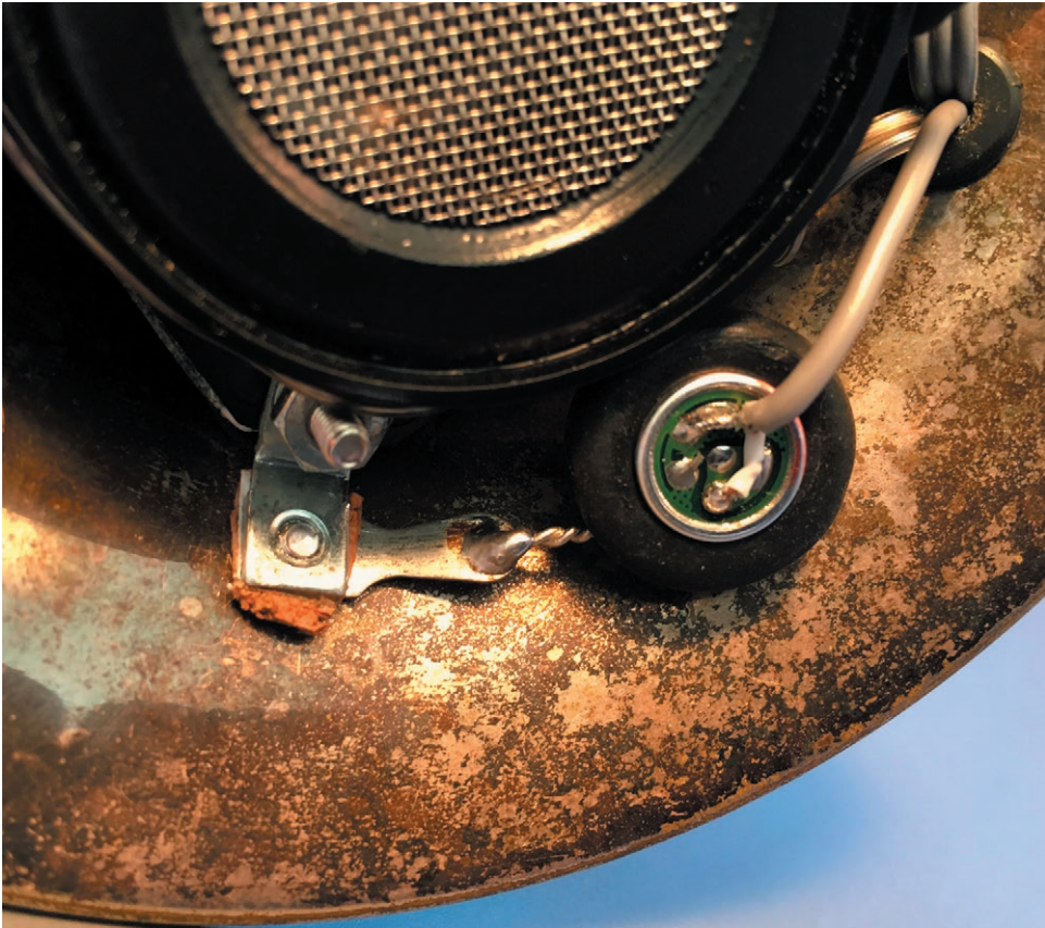
Figure 25. Pressure-zone electret microphone mounted inside bell.
