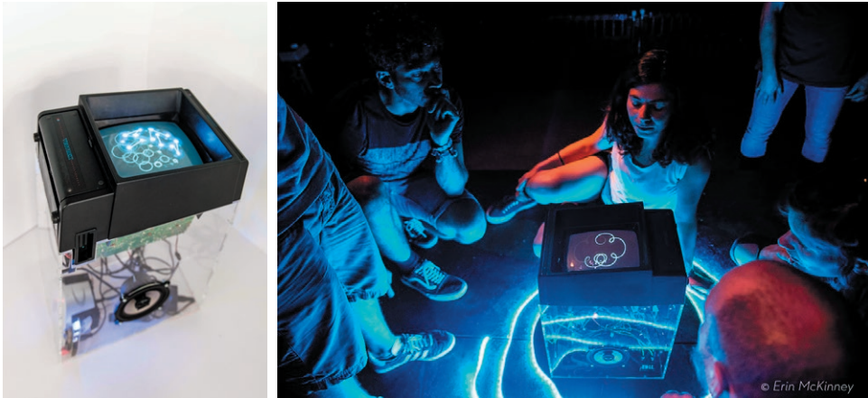
Figure 6. Celestial Harmonies - hybrid contemplative installation using a vector monitor from a modified Vectrex game console from the '80s, a Bela computing platform, speakers, and amplifying circuitry.
