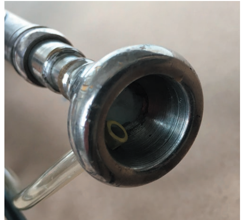
Figure 9. Air pressure sensor and hose coupling to mouthpiece.
