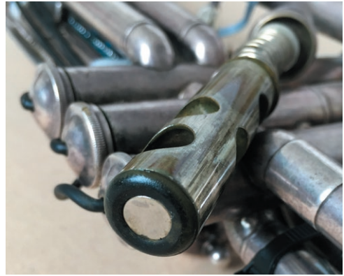
Figure 8. Valve sensor: Hall effect sensor (left), and magnet embedded in valve base (right).
