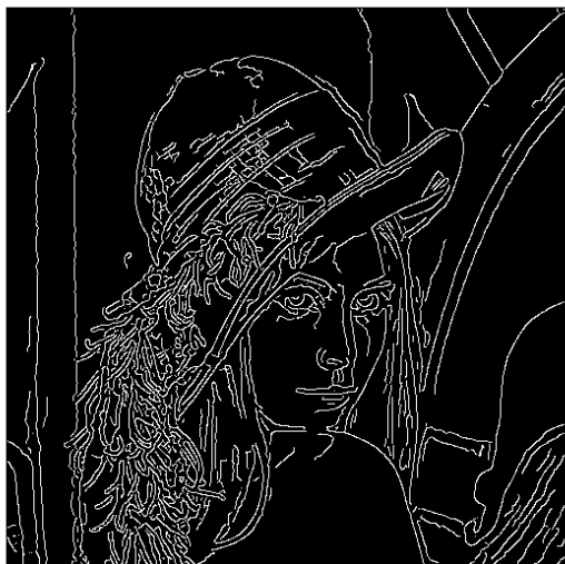
FIGURE 14. 512 x 512 edge detected of original image.
