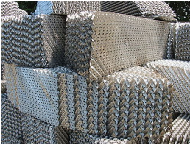
Figure 9. Photograph of structured packings (Wikimedia Commons, author: Luigi Chiesa).
