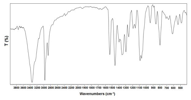
Figure 4. FTIR spectrum of compound 2
