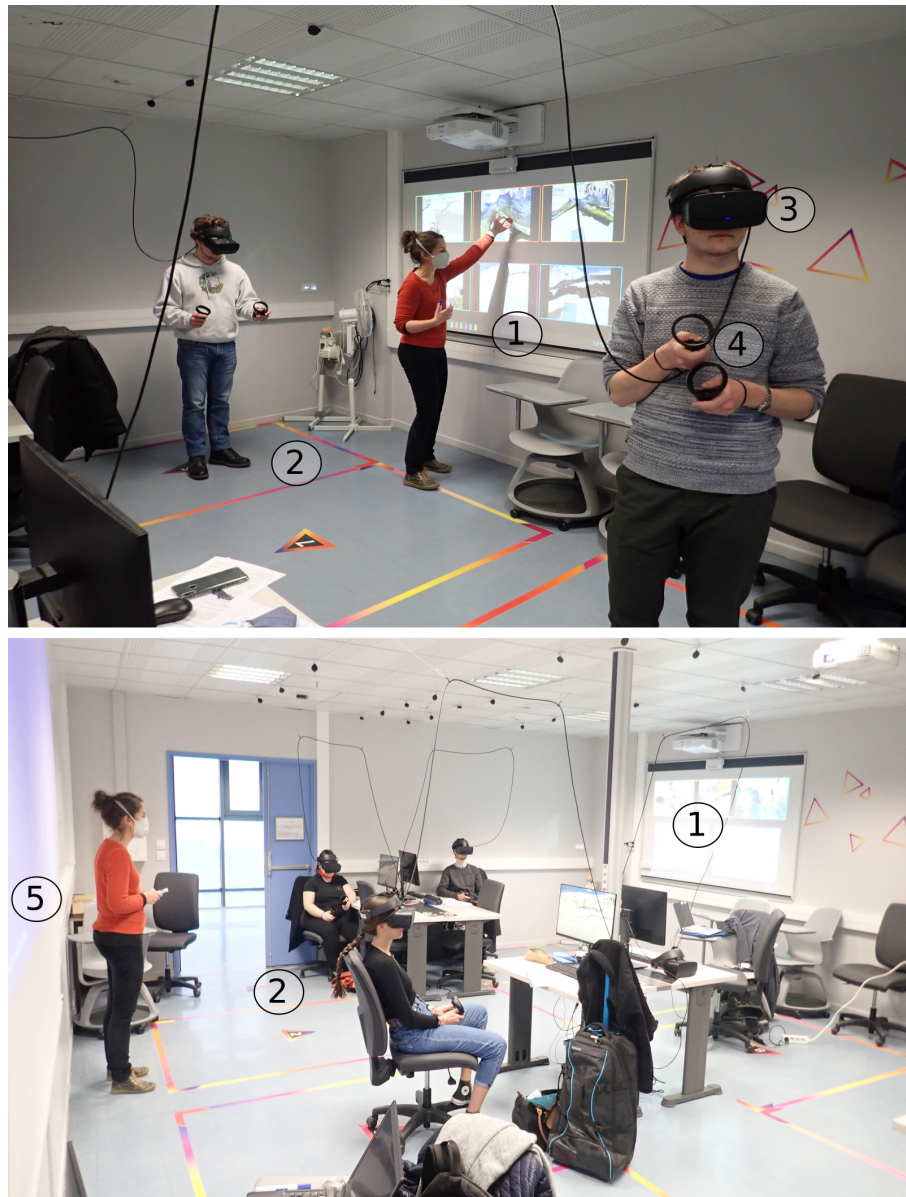
Figure 4. Views of virtual lab room in the alone in the field or single-user mode in which teacher (in orange) is outside the virtual environment. (1) Solstice collaborative screen-sharing system, (2) virtual box where limited real displacements of the user are allowed, (3) Oculus Rift S headset, (4) controllers, and (5) projection screen for teacher computer are all shown. It is worth noting that some students prefer to operate in VR while seated, while others find it more natural to be standing or moving within the limits of their virtual box (2).
