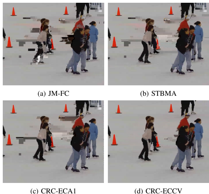
Fig. 12: Visual comparison of the literature methods to the proposed approach on AVC encoded Ice sequence (4CIF) at QP32 for an E_b/N_0 value of 8 dB
