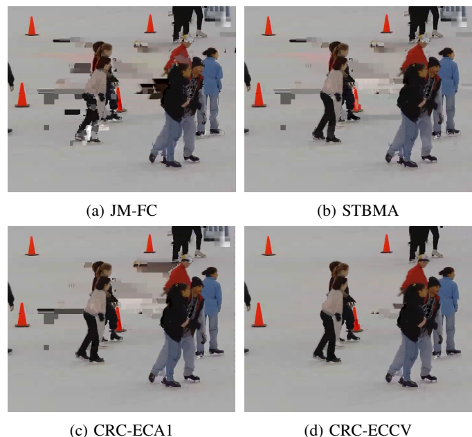
Fig. 12: Visual comparison of the literature methods to the proposed approach on AVC encoded Ice sequence (4CIF) at QP32 for an E_b/N_0 value of 8 dB
