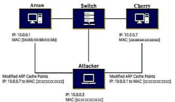
Figure 18: Address Resolution Protocol (ARP)
