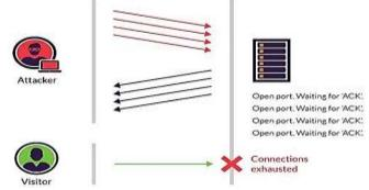
Figure 6: TCP SYN Flood Attack
