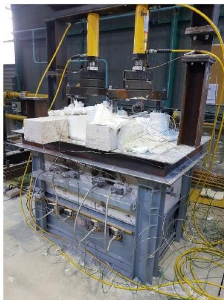
Figure 1: CSTB's furnace and loading system for fire tests on bonded anchors
