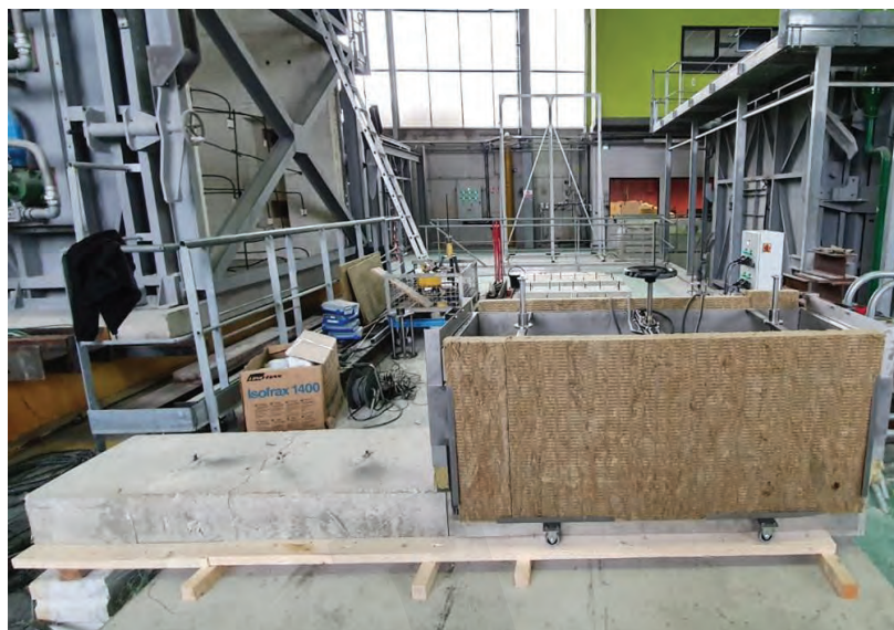
Figure 8. Heating system on top of a test slab in the fire resistance laboratory at CSTB.
