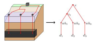
Figure 1: Representing a production network as a graph
