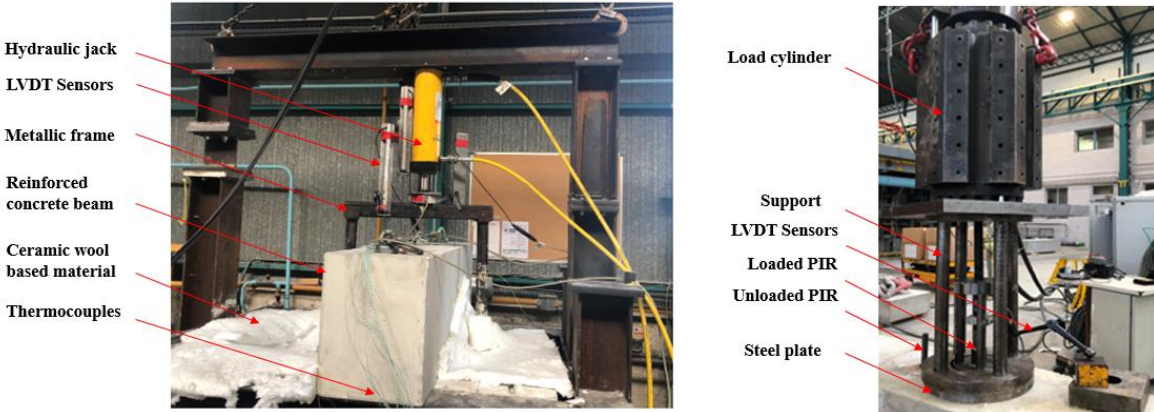
Figure 1: Testing apparatus in the heating phase (Left) and the cooling phase (Right)
